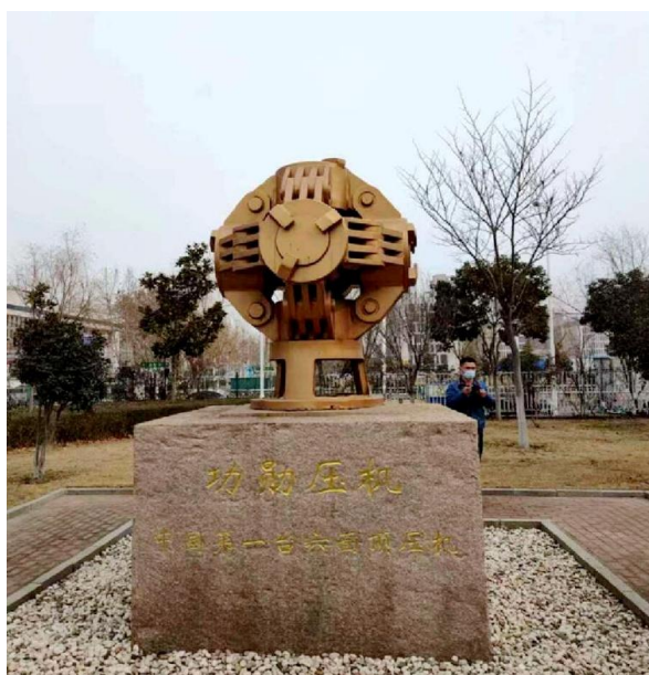
Fig. 3. The first six-punch press in China, the «DS-023» model, designed for synthetic diamond production [11]
