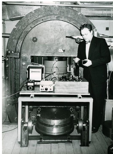
Fig. 1. Eric Lundblad at the Quintus press for diamond synthesis, 1953 (Quantis is the code name for ASEA's diamond synthesis technology development project, derived from the Latin word for «five», as diamonds have historically been considered the fifth element) [4]
